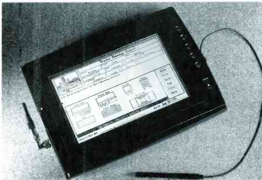
FIG. 1—THIS PEN-BASED PC from GRiD features wireless RF connectivity to Novell networks.
